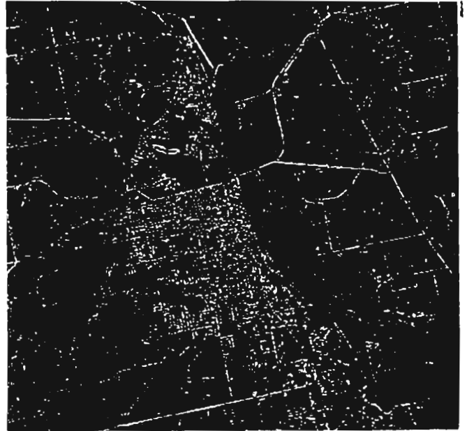
Fig. 8 (b) Initial road operator thresholded at 90%
