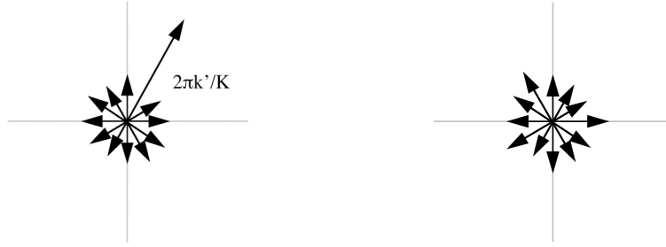
Fig. 2 Graphical depiction of LPCC filter response to a training image (left) and noise (right)
