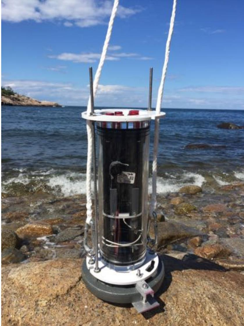
**Fig. 5 Ready to deploy with app running, lines attached and camera facing outward with a clear field of view.**
