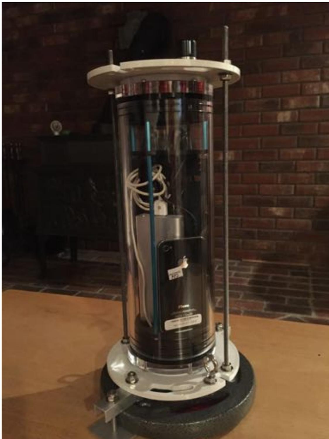
**Fig. 4 Assembled device. If you are using the camera make sure the iPhone camera is facing outward and has an unobstructed field of view.**
