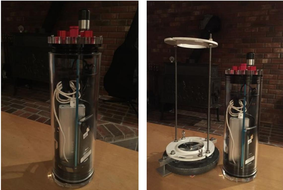
**Fig. 2 Watertight enclosure (left) next to deployment fixture (right). The deployment fixture holds the Aquipod in place by means of the two white PVC flanges.**
