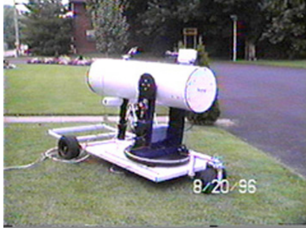
Figure 1 16" Newtonian telescope mounted on Scope Transport Unit.
