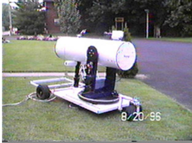
**Figure 1 16" Newtonian telescope mounted on Scope Transport Unit.**
