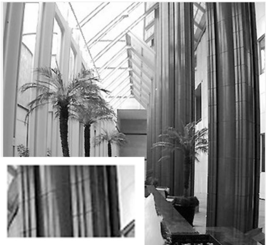
**Figure 4. Example of a wide-angle image. Curvature of columns and window frames is "barrel distortion" associated with the wide-angle lens. The inset at lower left demonstrates that the curvature caused by the lens cannot be detected over a small fraction of the image length. Photograph from reference ii.**
