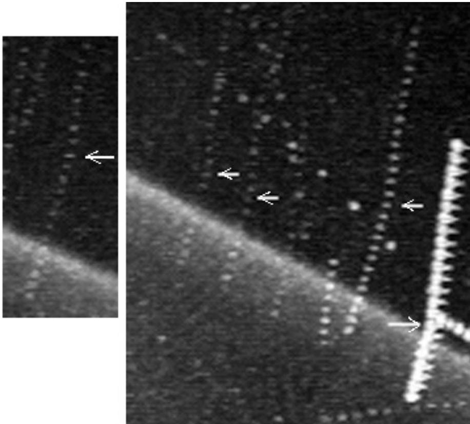
**Figure 7. An enlargement of a time exposure overlay using frames at 5-second intervals. Arrows indicate positions of five stars at the time of the light flash event. The positions of the stars at the point just above and 5 seconds prior to the light flash appear to fall closest to the intersection of the tracks before and after the thruster firing.**
